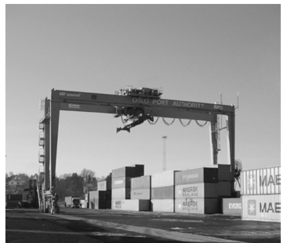
Figure 2: A Rubber-tired Gantry crane (courtesy of Kalmar Industries)
